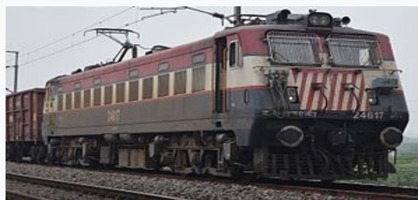
BHEL-made WAG7 of Erode Loco shed hauling freight
